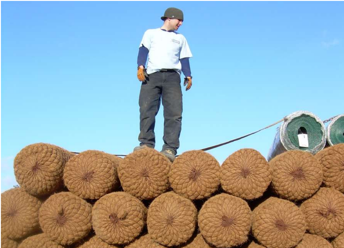
Image by G. Peabody. Coir are coconut husks wrapped in heavy fiber, wire or both.
