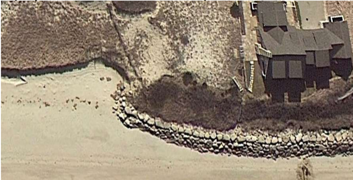
Image by Google Earth. Stone revetments may create “end scour” on adjacent property.
