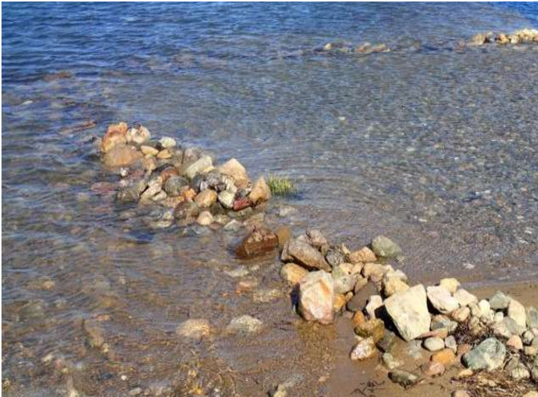
Image by G. Peabody. A temporary experiment: using piles of stones from the beach, with open spaces, to manage along shore tide current. Pointed in a "V" towards destructive storm fetch.
