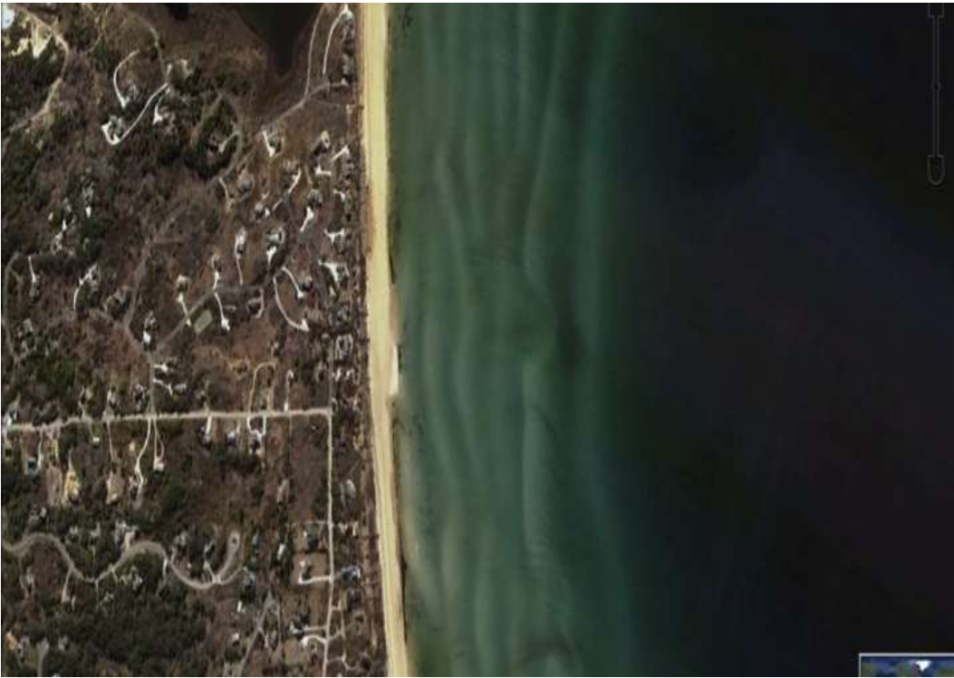
Image by Google Earth. Above image shows a near shore sandbar in a longshore Transit Corridor (path) of moving sand. Sand is transported over time, updrift to downdrift.
