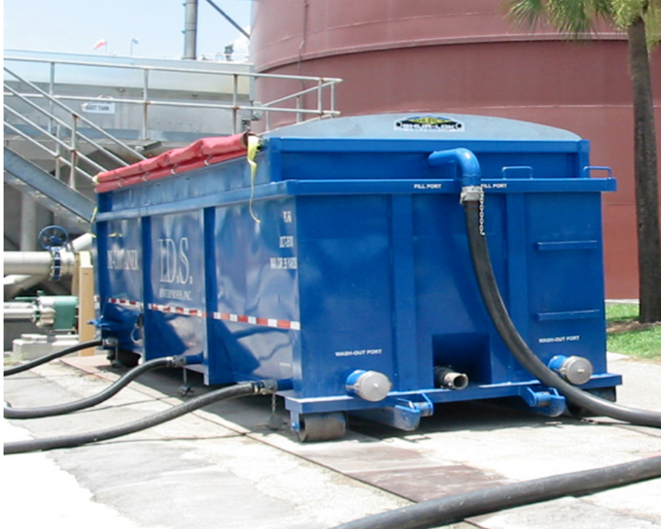
Settling tanks can aid in controlling pH and sediment
